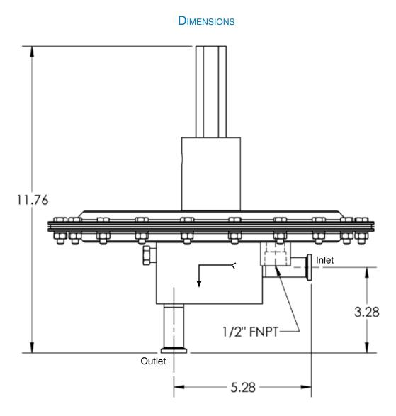
Note: Sensing line (not included) required to be installed per the Installation & Maintenance Guide for proper operation
