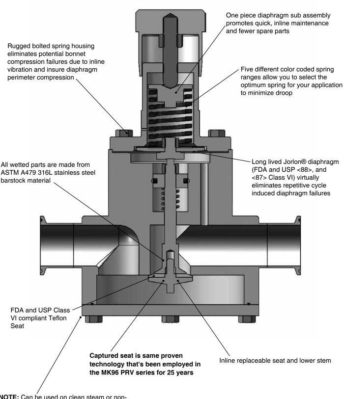
**NOTE:** Can be used on clean steam or non-cavitating liquids (the design is not drainable) with Steriflow engineering application approval.
