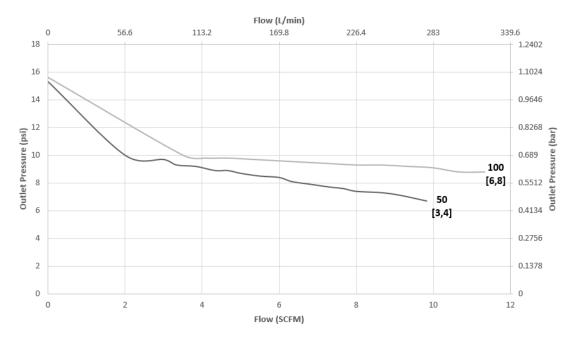
The graphs illustrate the change or "droop" in outlet pressures as the flow rate increases, and the lockup (setpoint rise) as flow decreases and approaches zero.
