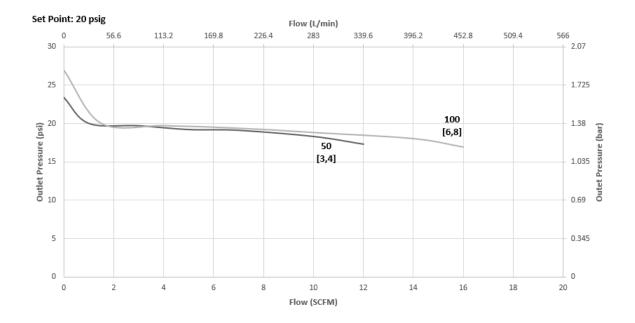
The graphs illustrate the change or "droop" in outlet pressures as the flow rate increases, and the lockup (setpoint rise) as flow decreases and approaches zero.
