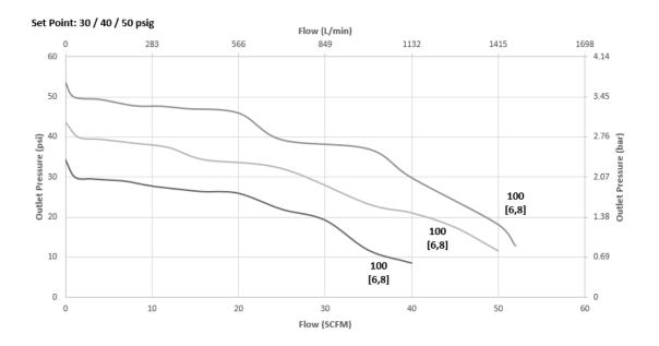
The graphs illustrate the change or "droop" in outlet pressures as the flow rate increases, and the lockup (setpoint rise) as flow decreases and approaches zero.
