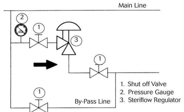
2. strainers at the valve inlet are not necessary.
