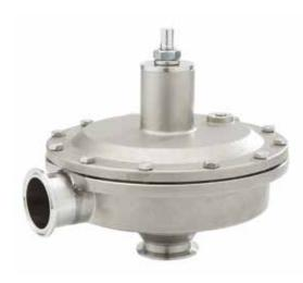
The FB5CPM (inlet) and FB6CPM (outlet) are air loaded sanitary constant pressure modulating valves, designed to allow the user to change set-points remotely via a cabinet or panel mounted air regulator, or through a distributed control system or PLC, using an I-P transducer. The valve is preferred in HTST/UHT Pasteurization, after Heat Exchangers, and Bottling Lines.
