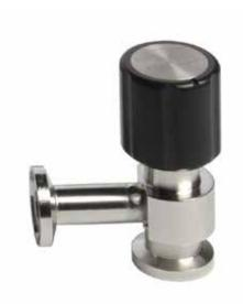
The SV Series was designed for use in high purity steam and culinary steam and water systems. The SV Series utilizes a steam resilient Perlast seat seal to ensure optimum service life and bubble-tight shutoff. Because of these design characteristics, the SV is also used for any general sanitary sampling application where a manual valve is required.
