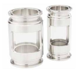
Inline tri-clamp, double window sight glass for media and purified water applications for the food & beverage and consumer health and beauty industries. Suitable for CIP and SIP, the SG Series has a large viewing area, full bore flow path, and a metal stop that provides ideal o-ring compression and prevents pipe torque from affecting glass.
