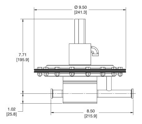
DIMENSIONS 1" JSRHULP SANITARY PRESSURE REDUCING VALVE F/ ULTRA LOW PRESSURE. 1" ASME BPE TRI-CLAMP ENDS
