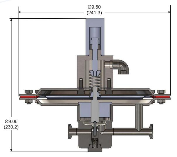
The JSRULP has very low set point capability, and impressive performance. Set points are between 3-18" wc [(0.11-0.65 psi), (7.47-44.79 mbar)]. Engineering also produced this compact valve with droop < 4 in wc (10 mbar), and maximum Lockup < .4 in wc (.1 mbar) across the valves complete operating flow range. Even though most pharma operating gas flow are very stable, this still gives Steriflow an edge of the competition, and a great selling point.
