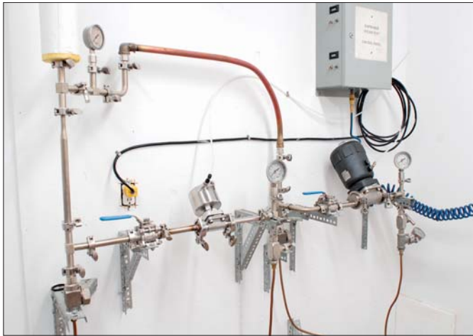
Steam cycle testing of Diaphragms
