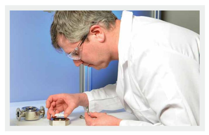
Biopharmaceutical process design engineers have rarely felt comfortable specifying "sanitary" spring check valves in WFI, buffer or direct process applications. The crevices, exposed springs, high particulate and cracking pressure with increasing differential pressure at increased flow, are just some of the reasons that spring and stem guided check valves are not used. Those are the specific reasons the SVC and SHC check valves were developed.
