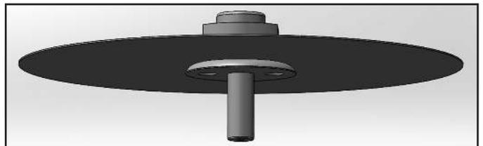
11. Replace range spring (12), spring seat (5), centering both on top of the upper diaphragm plate (4).
