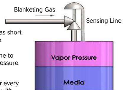
1. Make the sensing line as short and straight as possible.
