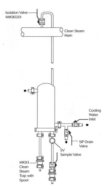
To ensure a representative steam sample is obtained, the steam feed should be taken off the top of the steam main or header as illustrated.
